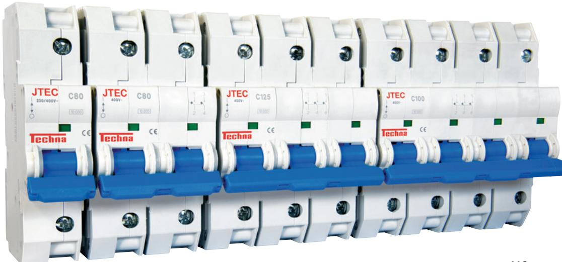
The Jtec 10kA High Current range comprises of three different ratings 80A, 100A & 125A and is available in 1-4 pole variants. These are all available in trip curves of B, C and D, providing a cost effective solution for larger current ratings. Due to the higher current ratings they are 27mm wide (1.5 modules) per pole.
